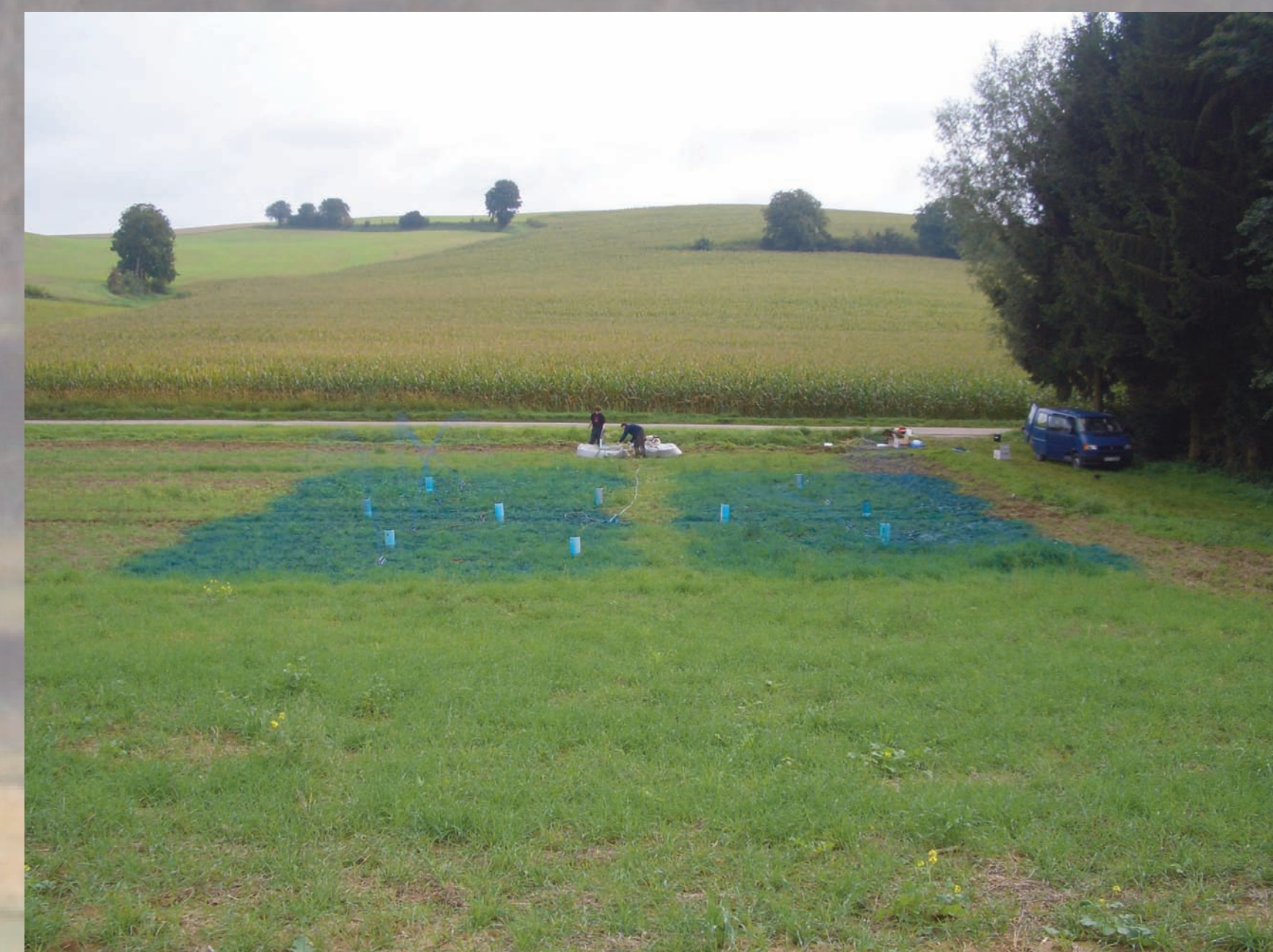
Fig. 2: Irrigation site after the application of the Brilliant Blue dye tracer. The plot is located approx. 15 m away from a brook and was monitored with 10 precipitation samplers.
