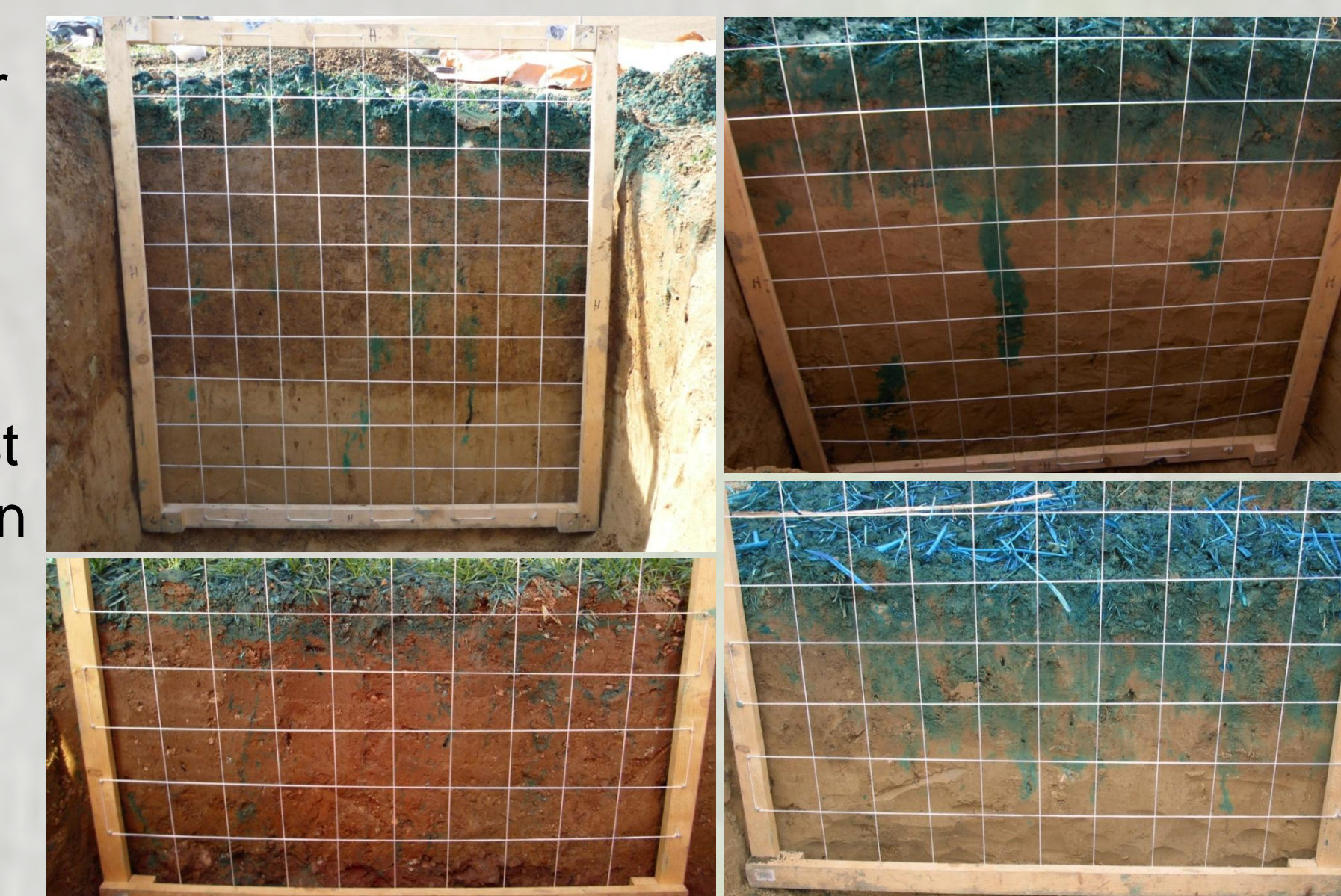
Fig. 6 Infiltration profiles showing a large variability in infiltration front at soil surface and infiltration from macropores to the matrix
