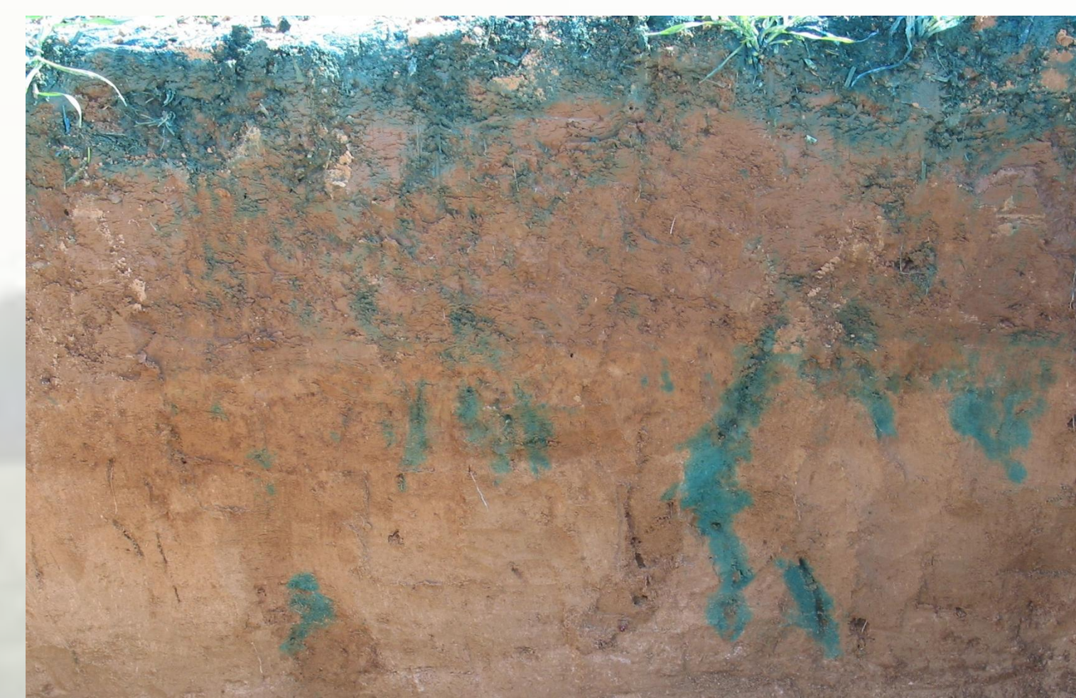
Fig 1. Dye-tracer infiltration pattern, with macropores
